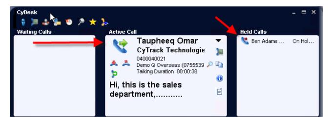
The user can toggle between the various calls by simply putting the active call on Hold by pressing the hold button and double clicking on the call they wish to take.
